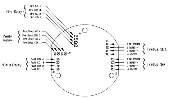
\* Fault relay is shown in the energized condition during normal operation (No Fault).
