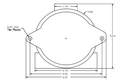
Figure 8: Model SS4-AS/-AS2 Detector Enclosure - Rear View
