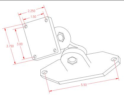
Figure 5: Model SM4 Stainless Steel Swivel Mount
