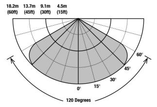
Figure 1: Field of View, Horizontal, and Vertical. Sensitivity to 1 Sq. Ft. Gasoline Pan Fire
