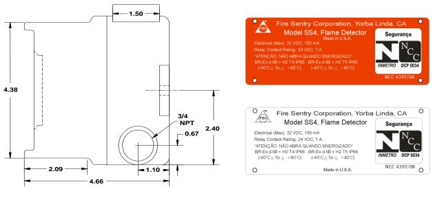
Figure 6: Model SS4-AS/-AS2 Detector Enclosure (Side View)
